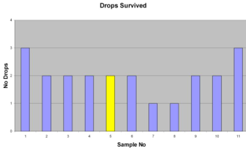
Marks on rope These did not seem to make any difference to the survival rating as the sample with the glaze is number 5.
