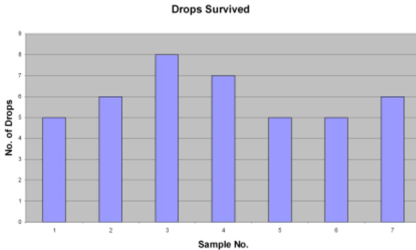
So we have a single length of rope with 7 samples taken at 30 meter distance along it. you can see that for what should be 7 identical pieces of rope, we found a variation in survivability of between 5 and 8 drops survived.
