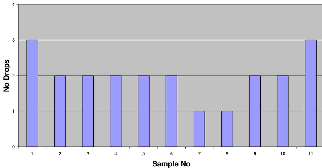
*Graph 2 - Showing the number of drops survived by samples of rope taken in sequence from a single 30 m piece of used rope*
