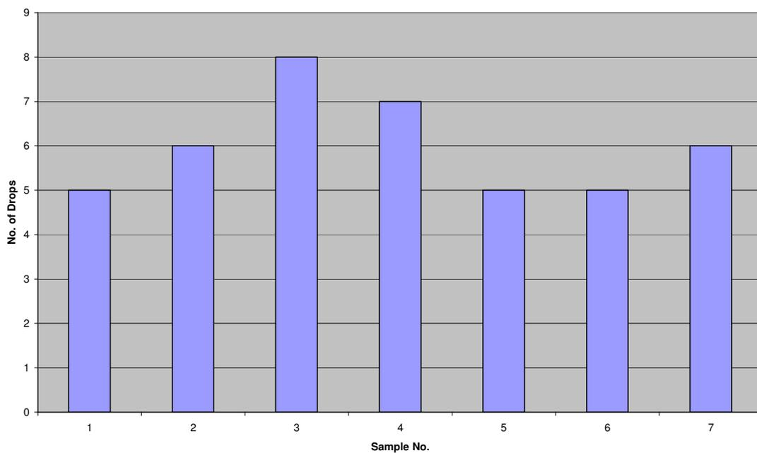
*Graph 1 - Showing the number of drops survived which the 7 samples taken from the same piece of new manufacture rope*
